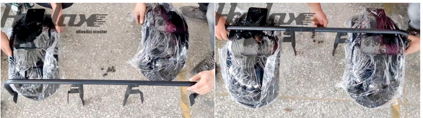
14: Place the fender in the bracket and tighten the screws.
