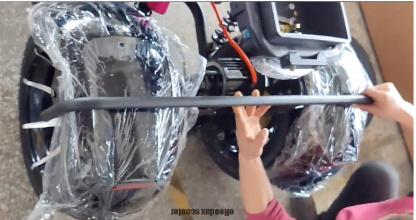
15: Install the installed fender assembly on the motor bracket
