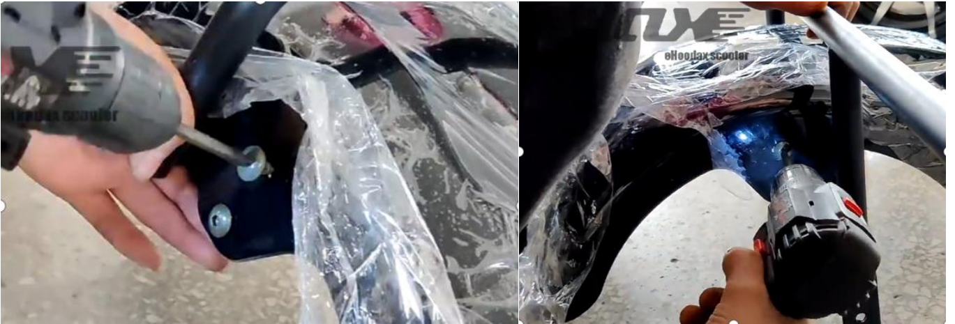
15: Install the installed fender assembly on the motor bracket
