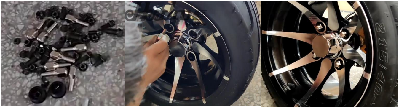
13: Put the tires on both sides on the motor, and tighten all the screws.
