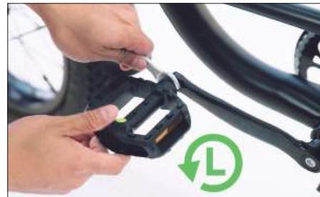
Thread pedals into crank arms following arrow directions (marked on cranks), then tighten with a pedal wrench.
