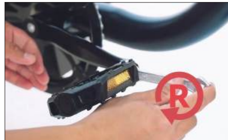
Thread pedals into crank arms following arrow directions (marked on cranks), then tighten with a pedal wrench.
