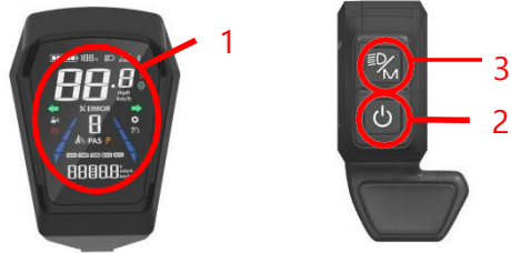
1: NFC Induction region 2: Power key 3: Light Switch / Mode Key
